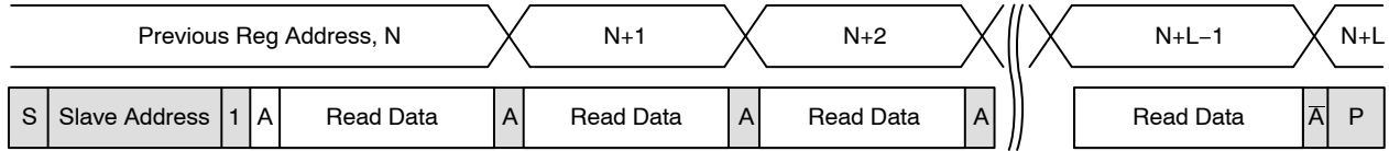
Figure 12. Sequential READ, Start from Current Location
